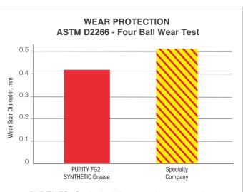
PURITY FG2 Synthetic delivers equal wear protection to a specialty lubricant suppliers' synthetic food grade grease. Less wear means fewer production upsets, higher productivity and lower maintenance costs.
